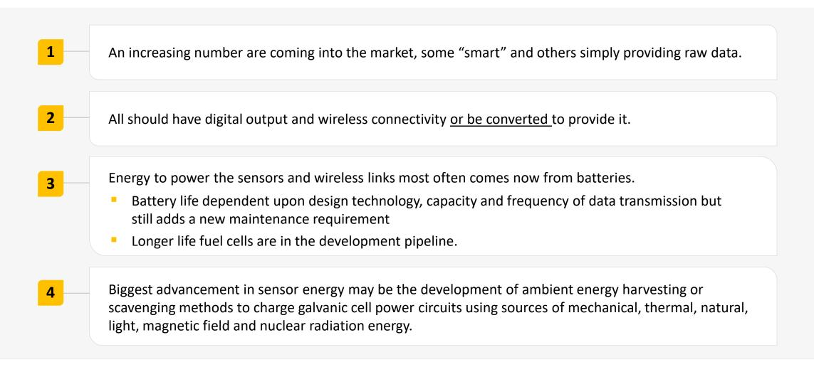
Source: Asset Condition Monitoring Management Chapter 10 pp170-171 provides more detail on battery alternative power sources for sensors.
