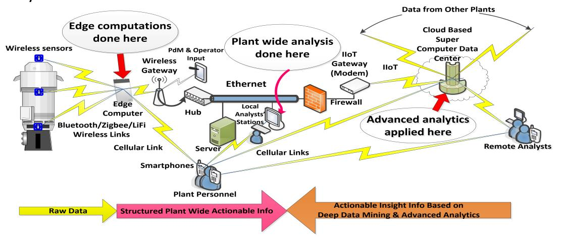
Unstated in the figure above is the possibility of moving beyond the actionable insight level possible with advanced analytics to <u>wisdom</u> about the plant being monitored.
