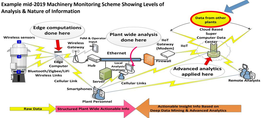
Comparable data from affiliated and unaffiliated plants that can be accumulated and used to hasten reaching conclusions about what is happening to equipment over time.
