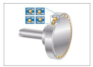
Looseness occurs when there is excessive clearance between parts. Looseness can occur in several places:
