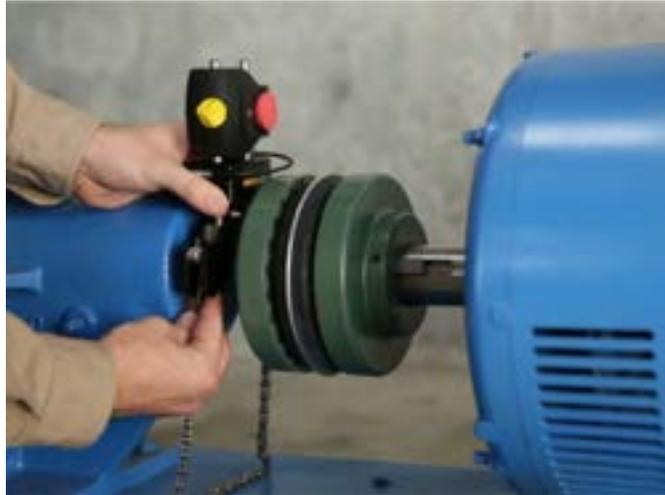
**1.** Mount Sensor on “Left machine” – usually Stationary - Mount as low as possible but high enough for beam to clear coupling flange
