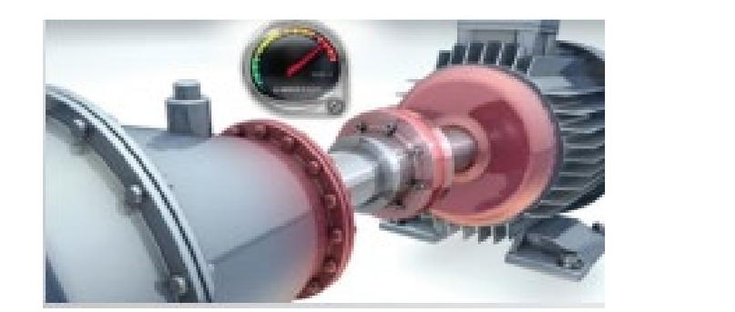
✓ Flexible couplings do not make up for the misalignment in a machine they simply transfer the forces to the bearings and seals causing rapid wear and failure
