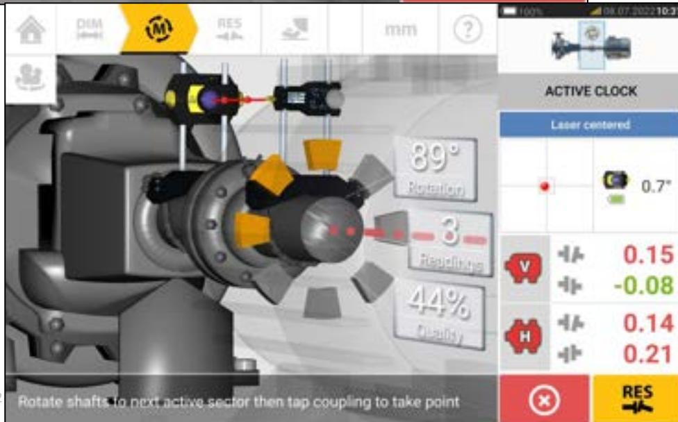
Once the set number of measurement points is attained, Tap **RES** to view machine foot results
