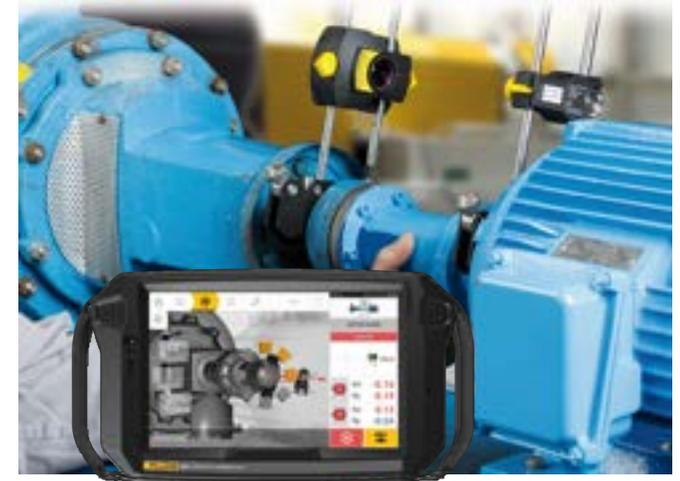
*"We electricians would replace the motor bearings and mechanics would replace the pump bearings and seals, and we'd slap it all back together. In a few months we would do it all over again. Then we learned to perform precision shaft alignments, and the bearings would last for years and years."*
