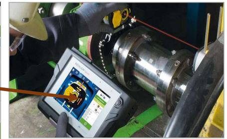
*“We electricians would replace the motor bearings and mechanics would replace the pump bearings and seals, and we’d slap it all back together. In a few months we would do it all over again. Then we learned to perform precision shaft alignments, and the bearings would last for years and years.”*
